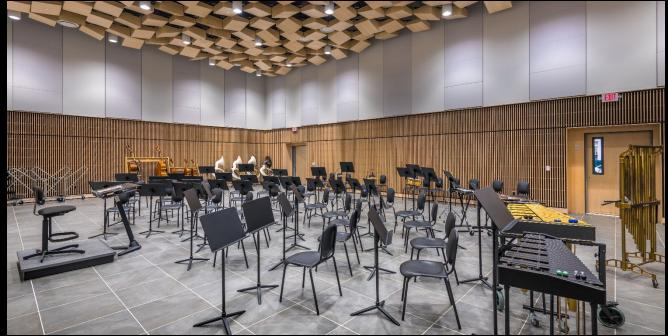
In the instrument rehearsal hall, dampening the sound of large ensembles is of paramount importance. As, a result the upper walls contain fabric wrapped acoustic panels dispersed evenly throughout.
